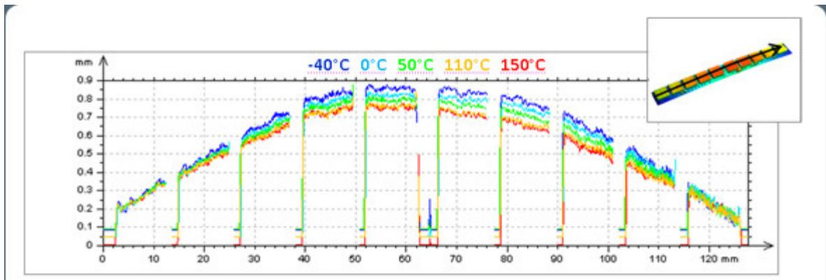
Both the strong overall warpage at all given temperatures as well as the important warpage variation with the temperature between -40°C and +150°C will certainly intrigue the reliability design engineer. The detailed analysis of the root causes will allow to decrease the overall warpage, and to reduce its temperature dependence, in order to finally enhance the in-field reliability of the assembly.
