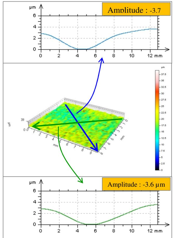
Fig. 3. Warpage measurement on the top die. The two diagonal 2D profiles are extracted, and their amplitudes are calculated. Amplitudes are marked with a negative (-) sign in case of concave profile shape, and with a positive (+) sign in case of convex profile shape.
