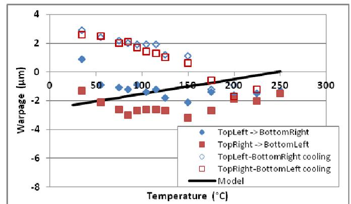
Fig. 11. Comparison of measured and calculated warpage in case of sample 3-a (thin bonded die with TSVs).
