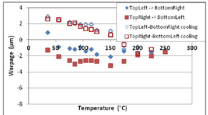
Fig. 7. Warpage measurement, sample 3-a
