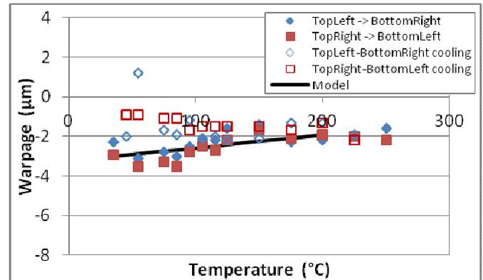
Fig. 10. Comparison of measured and calculated warpage in case of sample 1 (thick monolithic die).
