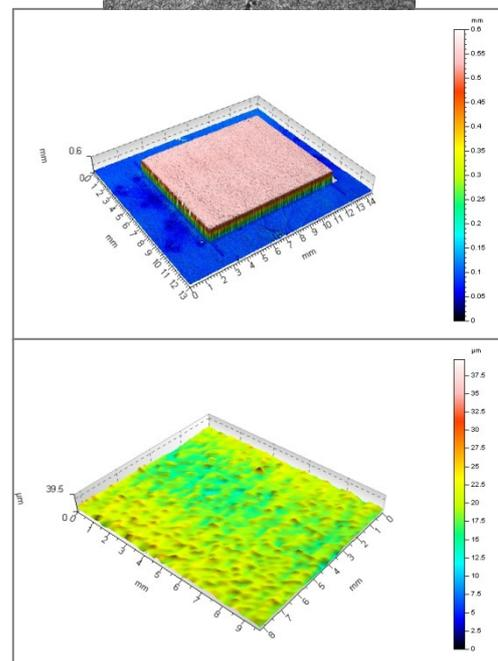
Fig. 1: Top: Photography of the PCB with the stacked die visible in the centre. Centre: 3D topography of the entire sample, obtained by TDM. The total depth of view (full color scale) is 0.6 mm. Bottom: Software zoom on the central die topography. The total depth of view represents 40 μm in this zoom view.
