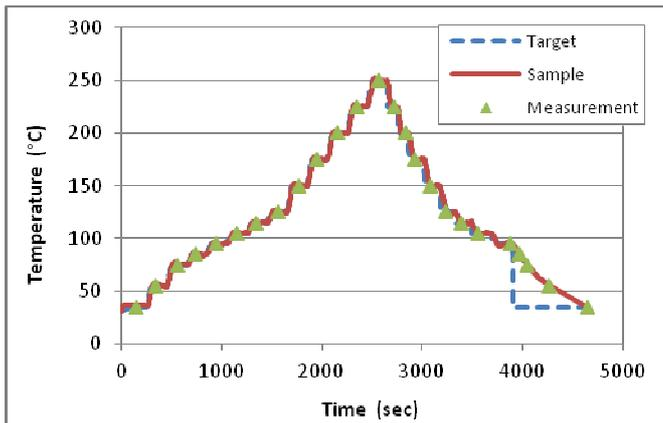
Fig. 2. Target temperature and measured temperature on the sample. The temperature is measured by a thermocouple, which is placed on the sample PCB at some mm distance only from the die.
