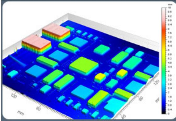
Topography of a 180×180mm assembly, at 220°C, acquired by TDM.
